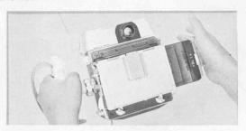
**Dry Plate** Size J  $(2\frac{\pi}{2} \times 3\frac{\pi}{4})$  dry plate is used in the plate holder which fits in the focusing screen holder.
